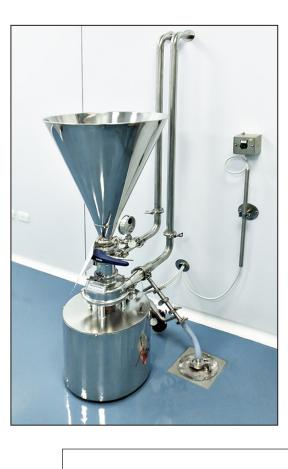
Frequently solid-liquid mixtures for IV solutions are be prepared through a sanitary triblender for a proper dosage of solid intake and liquid flow. The triblender basically consists of a casing and centrifugal-pump impeller with sanitary design, sanitary single mechanical seal, standard hopper clamp connections. The suction side has a double-wall tube that keeps the inlet of solids separate from the liquids, thus avoiding the formation of flocks before the material enters the casing.
