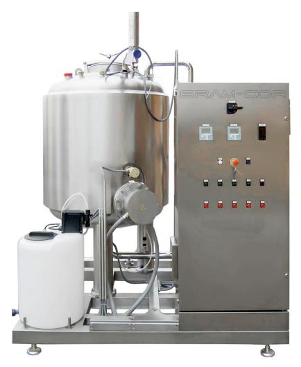
**BRAM-COR CLEANING IN-PLACE/STERILIZING SYSTEMS** are designed to fully meet cGMP requirements for cleaning and sterilizing practices commonly applied in pharmaceutical process tanks, lines and systems. Bram-Cor CIP/SIP systems are supplied as fixed stations or mobile skids with manual, semi-automatic or automatic control systems. Our CIP/SIP systems and be powered by electric heater, industrial steam, or combination units.
