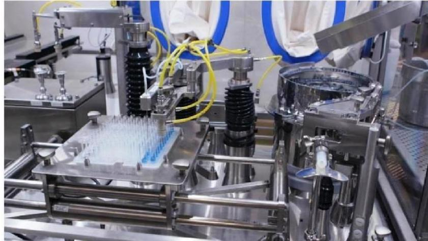
***M&O Perry Industries Liquid Filling and Stopper Inserting Machine for nested syringes, cartridges, and vials, Model NSCVF-L. Provides high accuracy fills 0.5% < 2% depending on container stability and liquid characteristics.***
