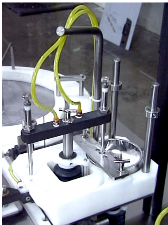
ACCOFIL® Powder Filling Principle Oscillating Needles
