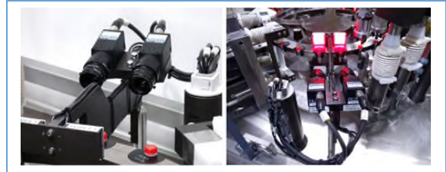
TORQUE STATION AND VISION INSPECTION
