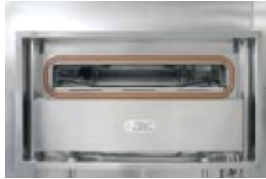
COOLING CHAMBER AIRTIGHT DOOR
